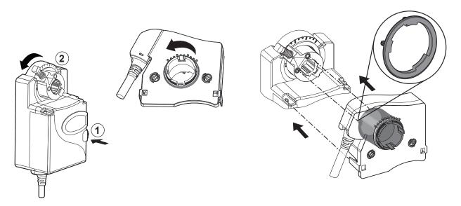
2. To remove the kit Place a screwdriver underneath the tab on each side of the actuator and firmly pull back the tab.
