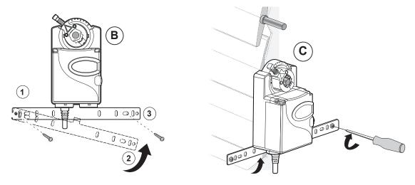
**6.** Apply power long enough for the actuator to travel a full stroke. Verify that the actuator rotates freely throughout the range.
