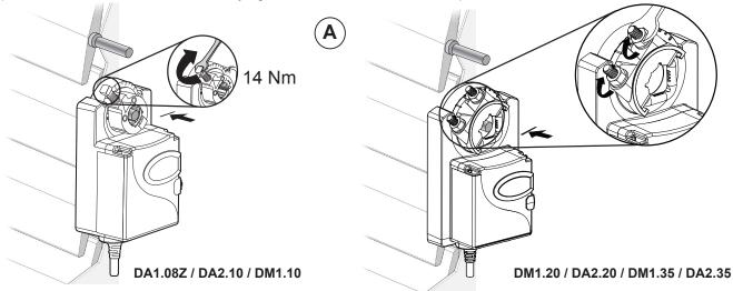
**5.** Lightly tighten one side of the anti-rotation bracket to the mounting surface. Swing the anti-rotation bracket under the actuator until it reaches the middle of the slot on the bottom of the actuator.
