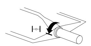
**2.** Bend or cut the anti-rotation bracket to fit the damper frame or duct as illustrated in figure below.
