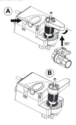
**5.** Reinsert the handle perpendicular into the actuator and tighten the handle screw.
