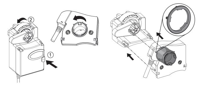
2. To remove the kit Place a screwdriver underneath the tab on each side of the actuator and firmly pull back the tab.
